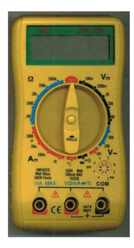
To use the meter as a temperature probe, put the red and black plugs in the holes shown, and set the pointer as shown ( $^{\circ}$ C). Avoid the hold button.
