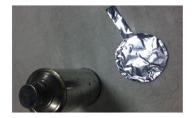
5. Working around the shape's perimeter, pinch the foil layers together and fold them under the shape by about an eighth of an inch (this keeps the layers together). It should look like the picture below. If you have enough scissors, students can make these shapes when they set up the system. It would be best to make one yourself ahead of time to serve as a model.
