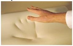
"Slow spring back foam" matches the pressure against it and slowly returns to its original form when pressure is removed. It is a silicone plastic with "open" cells (not closed bubbles). It returns to full size after being compressed. It makes comfortable pillows, mattresses, and surfaces on automobiles and motorcycles.
