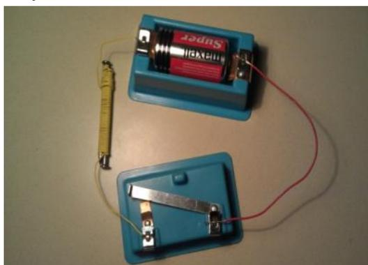
Connect the wires by depressing the clip, slipping the wire under the small hook, and releasing the clip.
