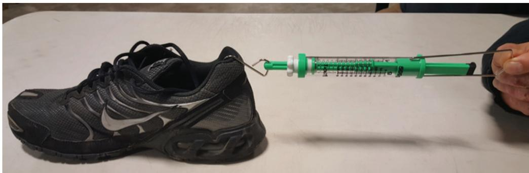
Hook the scale to the back of the shoe directly above the heel. Hold the scale so it is parallel to the tabletop and pull horizontally. As the shoe begins to move, record the force applied *at the moment the shoe moved*.
